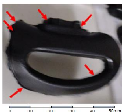
Figure 5 - Injected part with excessive flash
