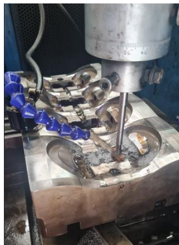
Figure 20- EDM operation in reworking cavities
