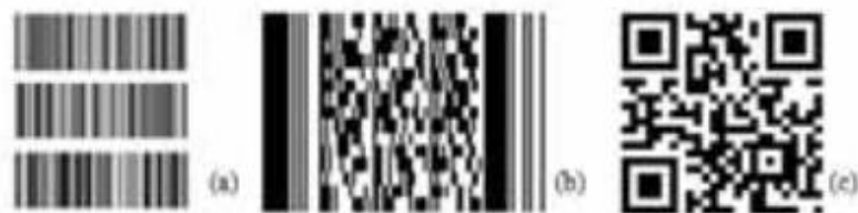
Fig. 2. Evolution of barcodes: (a) multiple barcode layout, (b) stacked barcode layout, and (c) matrix barcode layout.
