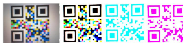
Fig. 11. Image Pre-processing a) Camera Image b) Filtered Image c) Color Estimation Of Cyan and Magenta
