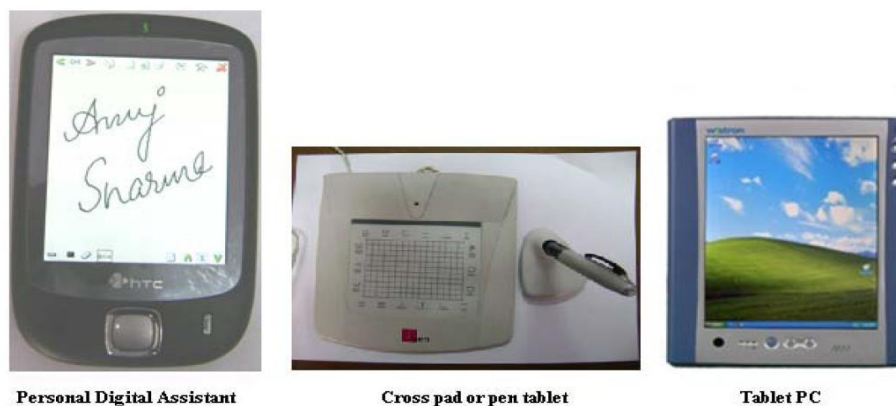
Fig. 2: Commonly used hardware devices for capturing handwriting.
