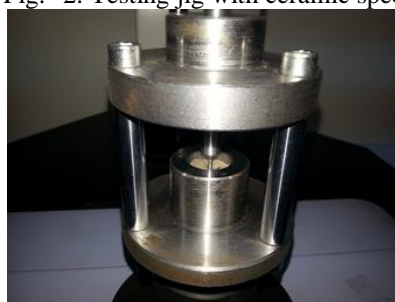
"Fig." 2. Testing jig with ceramic specimen
