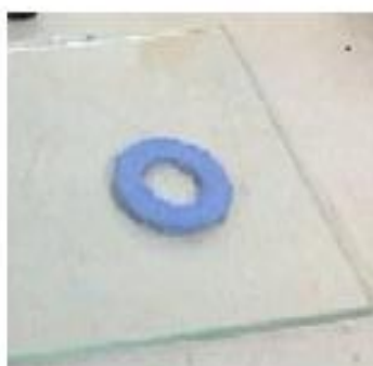
Figure 1: rubber mould used to make specimens
