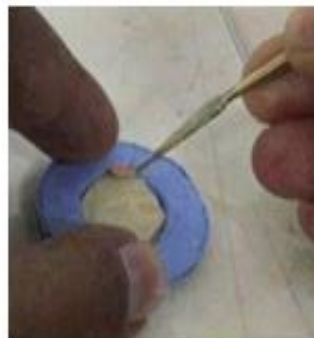
Figure 2: composite being packed into the mould
