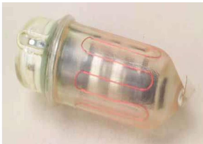
Figure 4. The wireless motility capsule (Saad, et al. , 2011)
