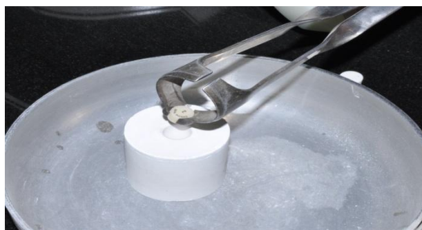
Fig 8 Ceramic ingots being placed in mold after preheating in furnace
