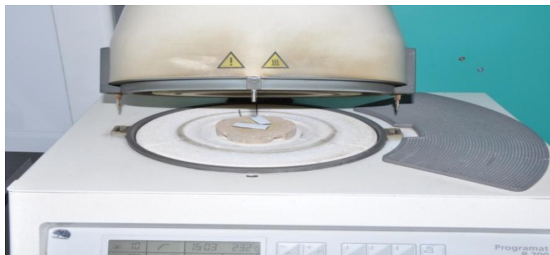
Figure 4. Metal strips place in furnace after adding opaque porcelain
