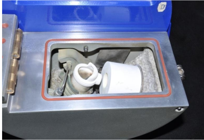
Figure 2. Crucible and mold placed in casting machine
