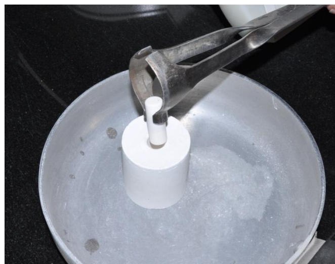
Fig 9 Plunger placed into mold for pressing in the pressable furnace
