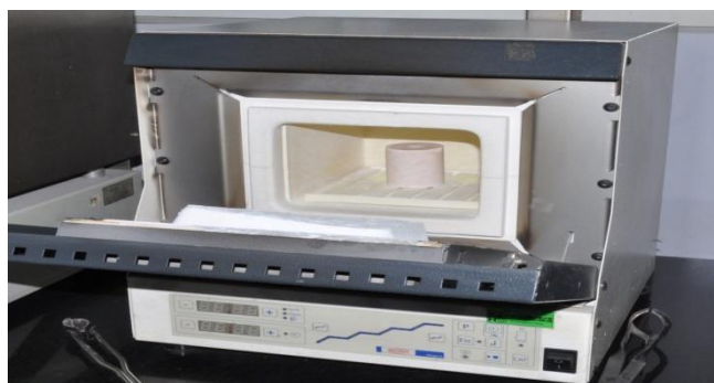
Fig 6 Mold placed in pre heating furnace
