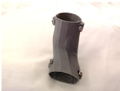
Fig-5: The 3D printed orthosis made of PLA plastic. It consists of the anterior and posterior parts, held together with metal screws.
