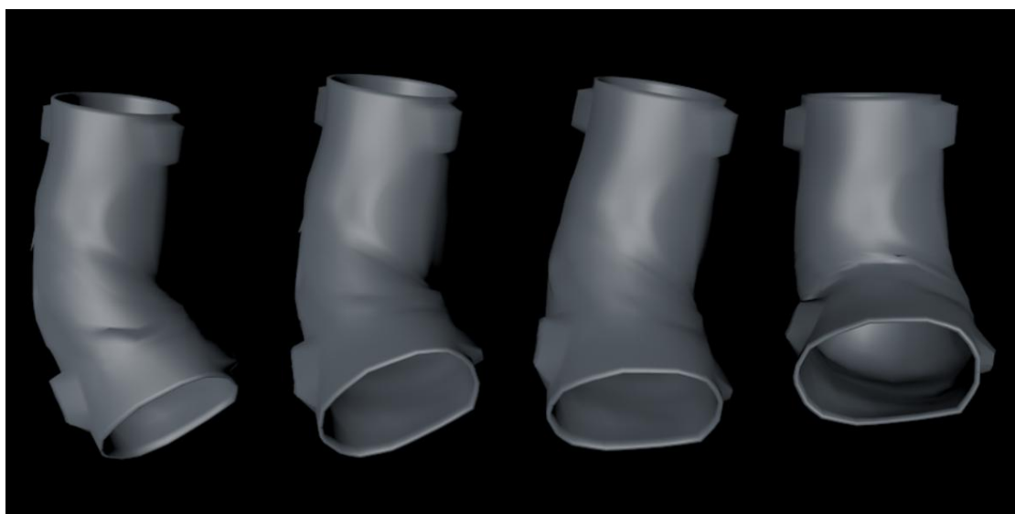
Fig-4: Model of orthosis is generated based on the computer model of the leg
