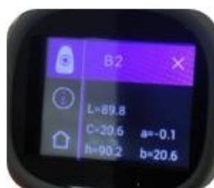
Fig 6. L*a*b* value on VITA Easyshade spectrophotometer.
