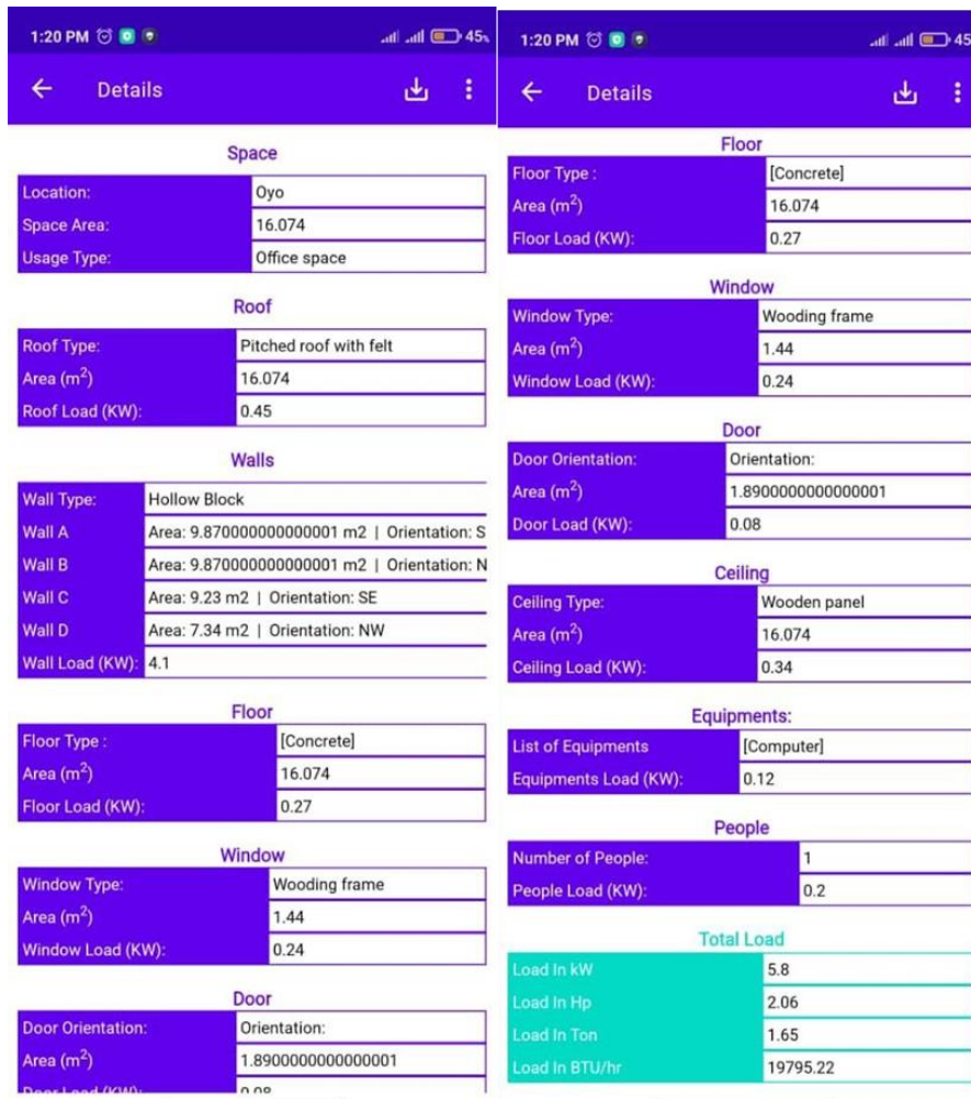
Figure 4: The software’s result output interface showing the generated result for the estimation.
