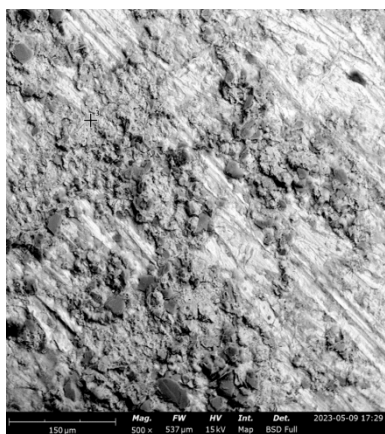
Fig11(b): SEM image and EDX analysis of mild steel after immersion in 1M HCl Blank solution
