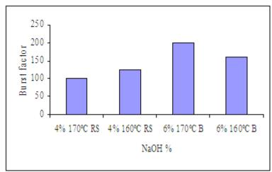
Fig(4): Effect of pulping temperature on burst factor of rice straw and bagasse pulp.
