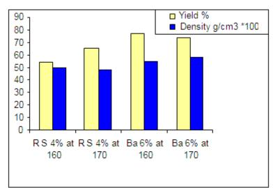
Fig. (1): Effect of pulping temperature on the yield and density
