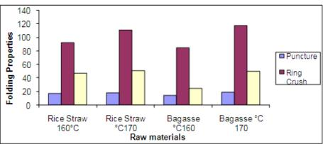
Fig(5): Effect of pulping temperature on folding carton properties.
