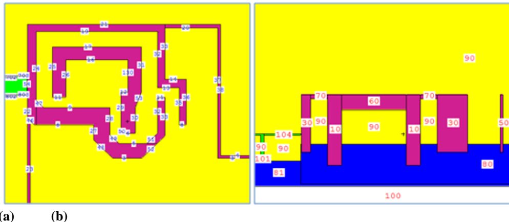
Figure 4: MCNP model (a) XY section with surface numbers and (b) XZ section with cell numbers.
