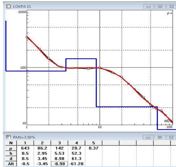
Figure 12: Showing curves generated for VES location 11
