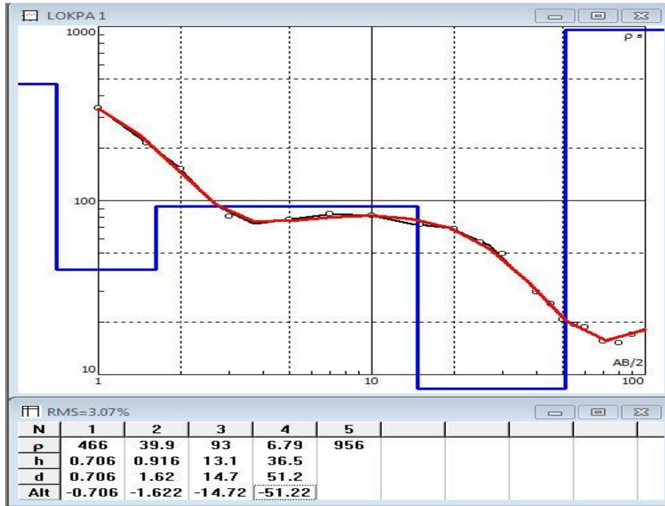
Figure 2: Showing curves generated for VES location 1
