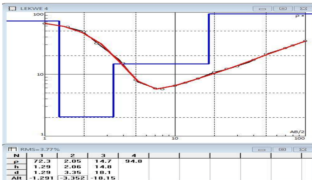
Figure 6: showing curve generated form VES location 4
