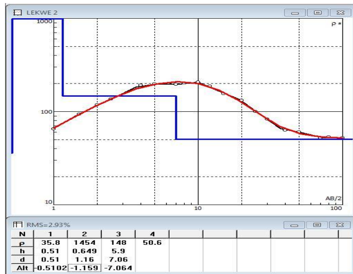
Figure 4: showing curve generated for VES location 2
