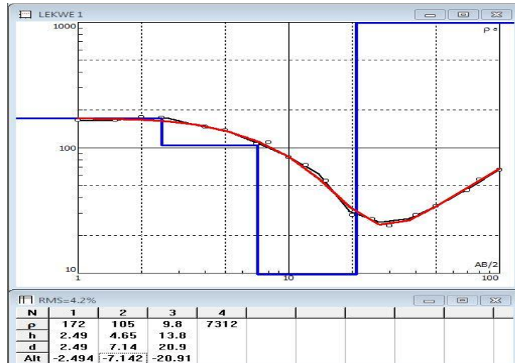
Figure 3: showing curve generated for VES location 1
