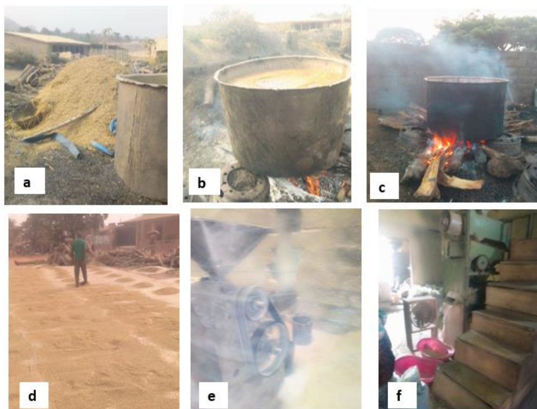
Fig. 1: (a) Chaff removing site (b) Parboiling site (c) Final heating site (d) Sun drying site (e) Husk removing/milling site (f) De-stoning site
