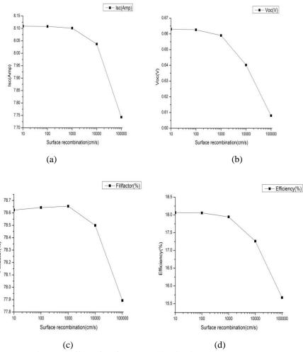
Figure 2: Effect of surface recombination in cell parameters
