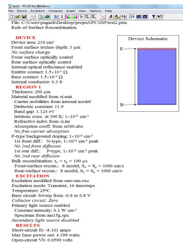
Figure 1: summary of simulation parameters for PC1D model.
