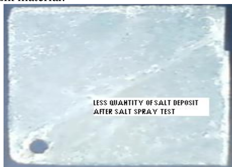
Fig 6: Showing the image of salt spray test on ZnO nanocomposite coating on mild steel sample.
