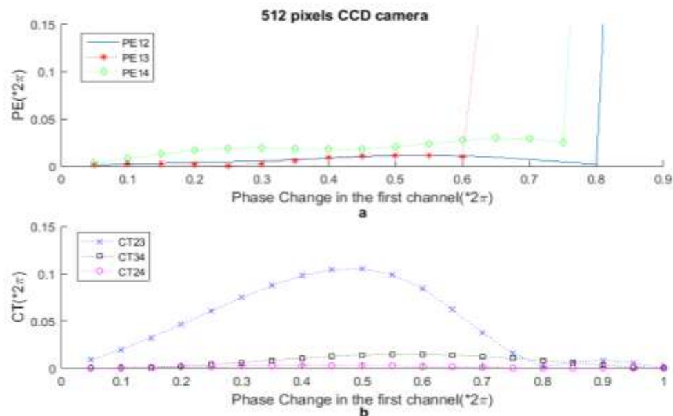
Figure 2 a) PE and b) CT dependence from the phase change in the first channel for a CCD camera resolution of 512 pixels
