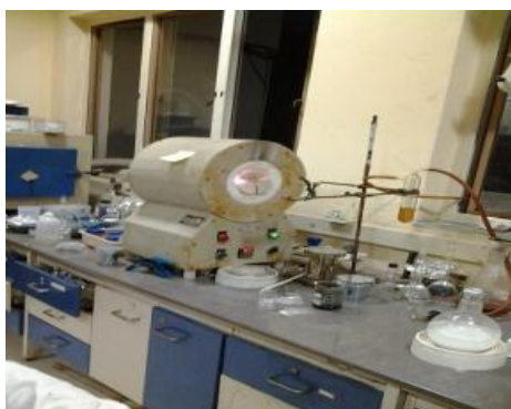
Figure 3 The cylindrical furnace, with precise temperature control N.C.L., Pune, India. The axial placement of the sample facilitates uniform regulation of the temperature
