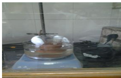
Figure 2 Oil bath & magnetic stirrer cum heater, with precise temperature control and provision for monitoring the number of revolutions per minute. The outer trough contains the oil whose temperature is maintained. The inner beaker contains the Nano material being synthesised
