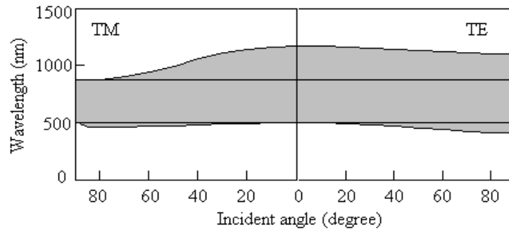
Fig. 6 PBG structure of combination of Fibonacci quasi-periodic structure and periodic structure
