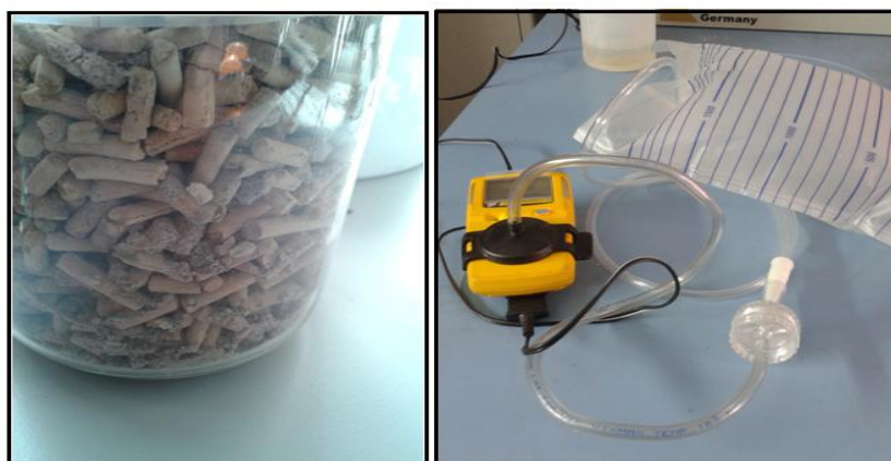
Figure 2. Commercial fixed bed column after passing raw biogas (Left); H 2 S gas analyzer connect to collected biogas bag (Right).
