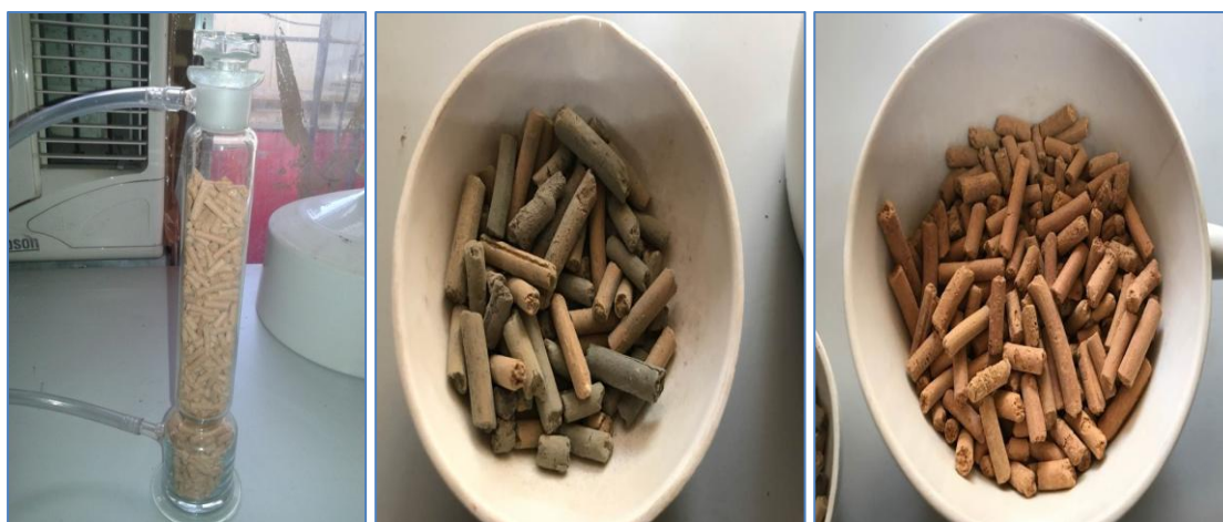
Figure 3. Iron Oxide filter media before and after passing raw biogas.
