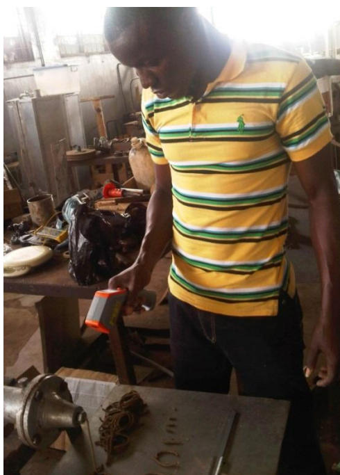
Plate 1: Pictorial view of one of the extrusion process while taking barrel temperature
