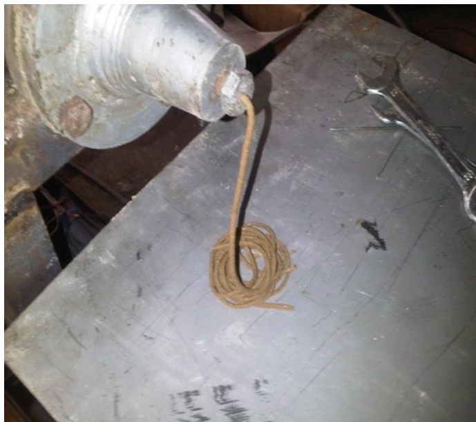
Plate 2: pictorial view showing extrusion of extrudate from the extruder
