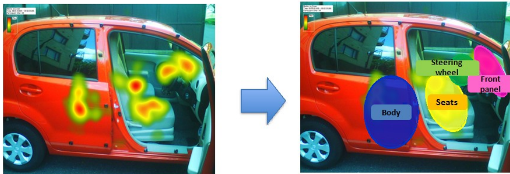
Fig. 4. The result of analyzing the time that eye sight resided on a particular part in eye camera
