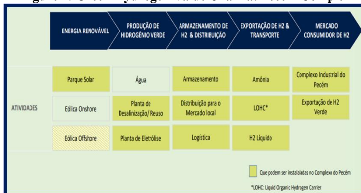
Figure 1: Green Hydrogen Value Chain at Pecém Complex
