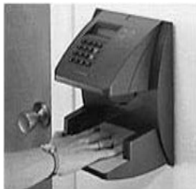
Figure 6: Hand geometry scanner [5]
