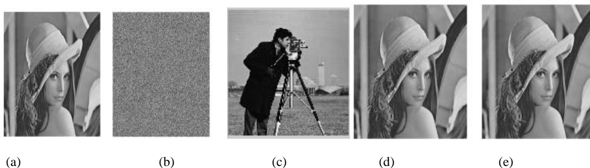
Figure 4. (a) original image, (b) encrypted image, (c) cloak image containing marked encrypted image, (d) decrypted image containing messages, (e) recovery version.
