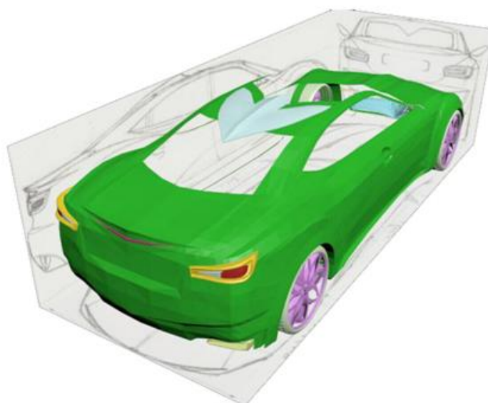
Fig. 3: Construction of body 3D model on the base of sketches
