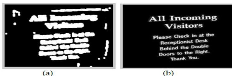
Fig.5. (a) Image after morphological operations, (b) Output image after segmentation.
