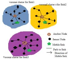
Figure.5. AVRP creates the anchor-based Voronoi scoping in an mWSN with three mobile sinks.
