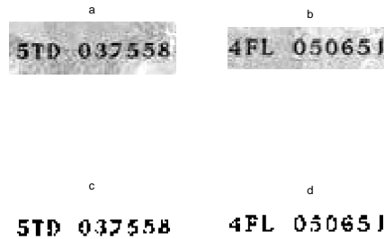
Fig. 3. Preprocessed serial number images: Original images: (a) and (b), Images with uniform background: (c) and (d).
