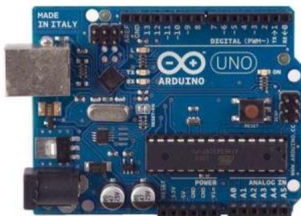
Figure 3: Arduino Uno board with Atmega microcontroller
