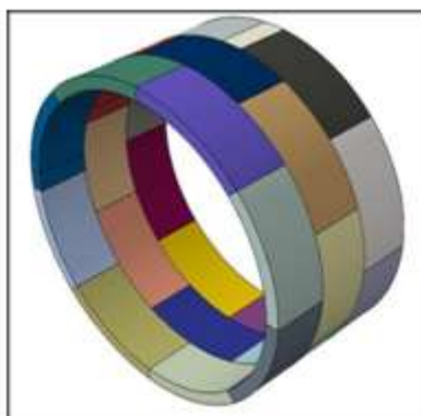
Figure 1. Staggered concrete segment tunnel lining
