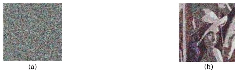
Figure 16 : (a) Ciphered scrambled image submitted to JPEG compression with quality loss of compression 100 and (b) the corresponding deciphered image
