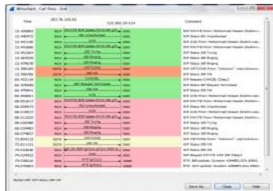
Fig.8 Flow graph of SIP register request from the host 203.76.105.82 to SIP server 123.200.24.214
