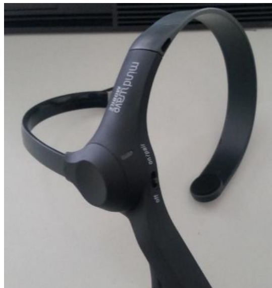
Figure2: Mind wave mobile equipment used as EEG sensor.
