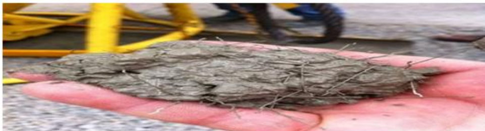
Fig.(5) Concrete mixture with 1% steel fiber
