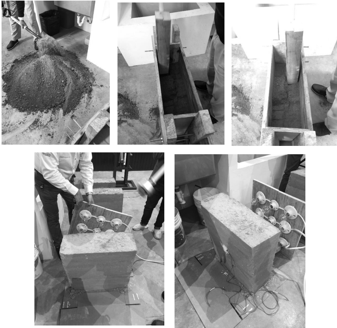
Images 3, 4, 5, 6 and 7. Soil screening stabilized with lime, tamped down, heat source colocation and thermocouples. Photo: Gloria Esmeralda del Angel Cavazos. Architect.
