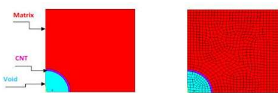
Fig.3.a Geometrical model at 2% volume fraction Fig.3.b FE meshed model at 2% V_{cnt}
