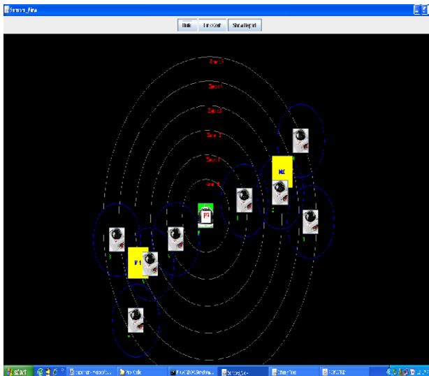
Figure 2.3. Mobile Agents moving along the tree path to collect the data from the sensors
