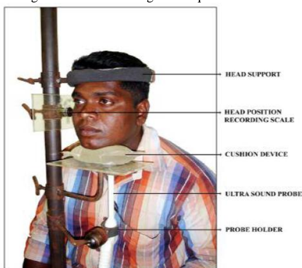
Fig 5: Cushion Scanning Technique with transducer
