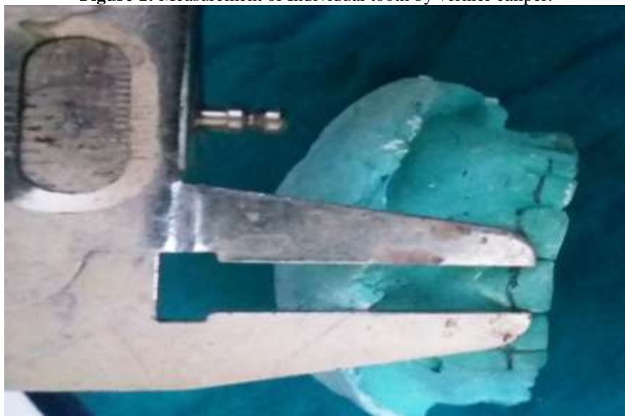
Figure 1: Measurement of Individual tooth by vernier caliper.
