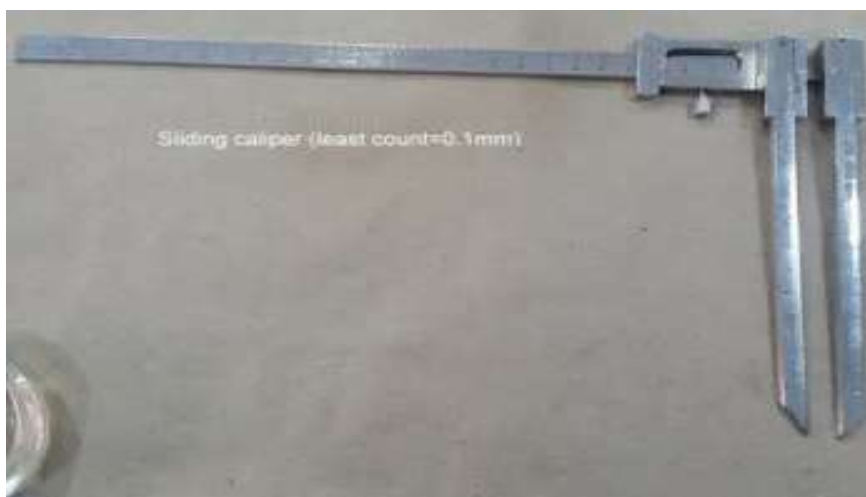
Fig-1: Slide callipers used for measuring distance of mental foramen from various landmarks
