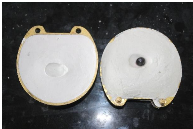
Figure 13: Dewaxed flasks (with corneal button in the correct position) ready for packing
