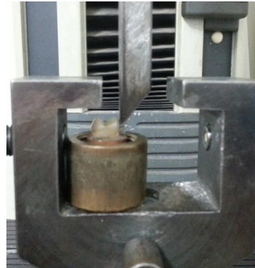
(Figure 6): Measuring the shear bond strength of the bonded bracket sample in the universal testing machine
