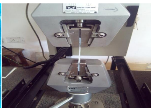
Figure 3. Specimen without intrinsic pigmentation stretched in the universal testing machine (Instron corporation 3382).
