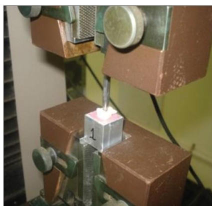
Fig.2 Loading of the specimens in the instron universal testing machine
