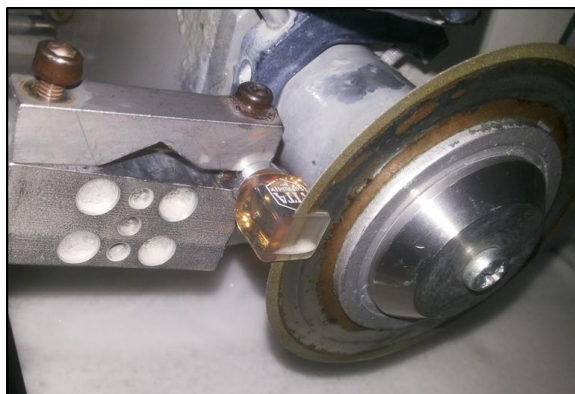
Fig. 1. Isomet disc used in sectioning Vita Suprinity block
