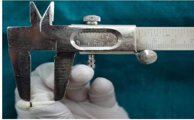
Fig.3: standardization of the sample at 12mm by using vernier caliper
