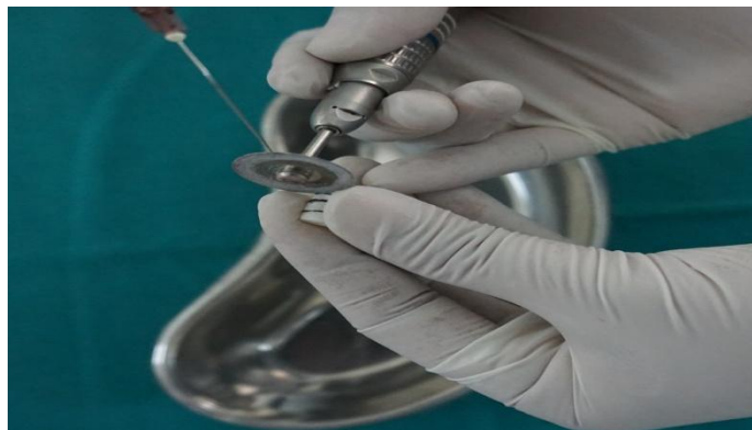
Fig.14: Sectioning of sample done at 3, 6 & 9mm
