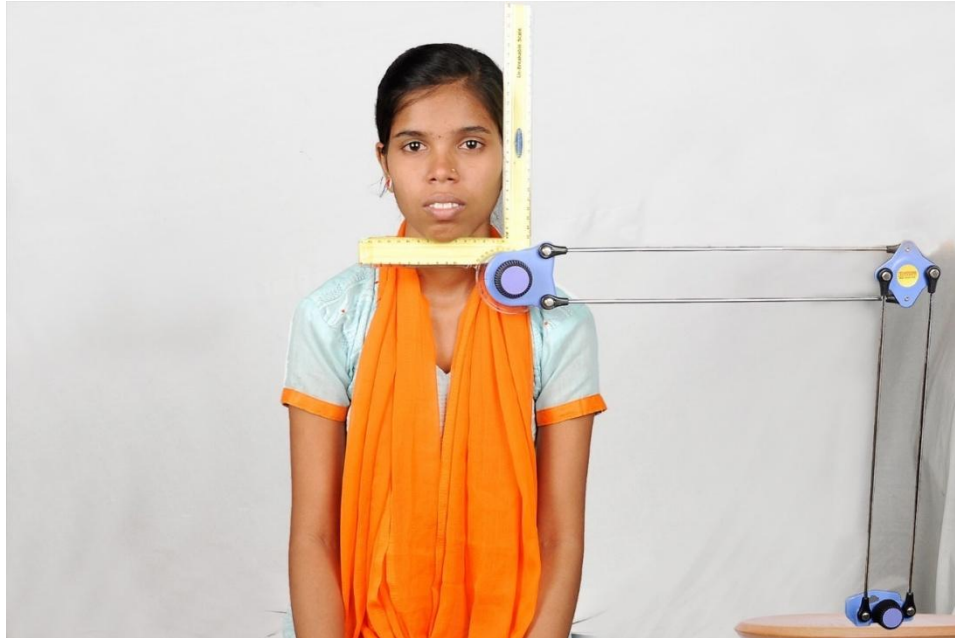
Figure shows position of patient and drafter (Technosigmaminidrafter) during frontal facial photography.
